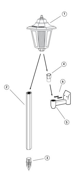
A flathead screwdriver is required for mounting the wall bracket.
